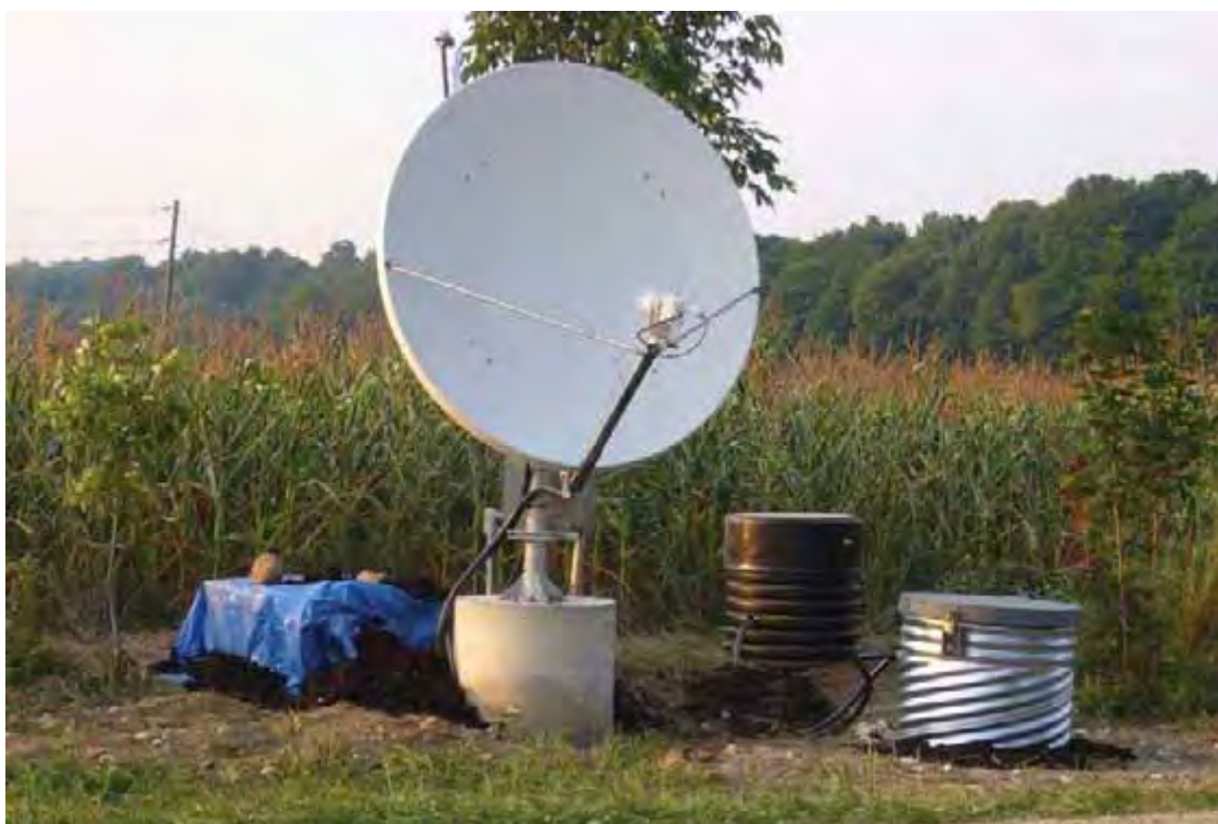
Low level seismic monitor
