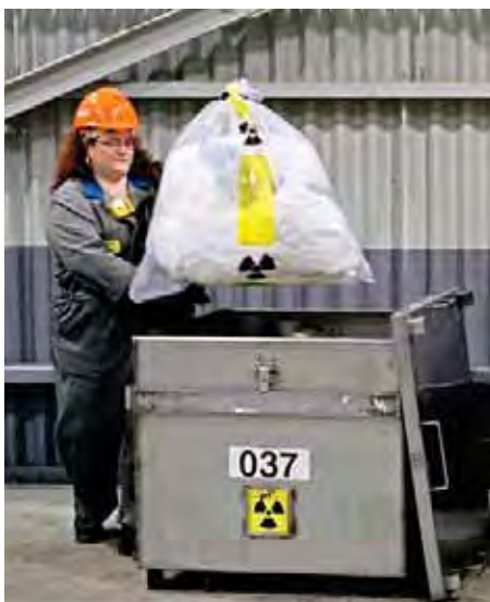
Low level waste at the WWMF is handled by trained personnel before processing by either incineration or compaction.
