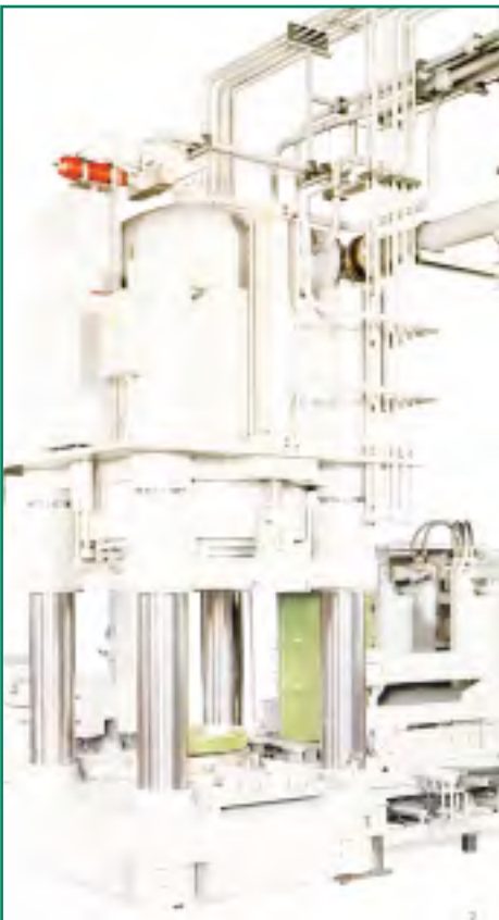
Super-compactor showing how much a drum (green) can be compacted.
